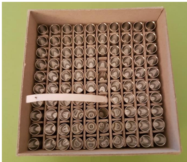
Figure 8.14: RFID tag inside aluminium shell positioned in the middle off 100 aluminium shells
