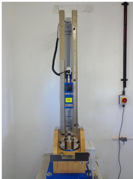
Figure 4.34: Julius Peters impact sensitivity apparatus
