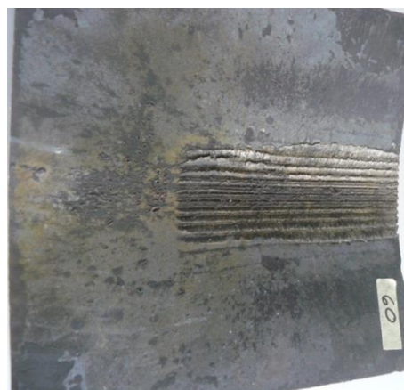
Figure 7.6: Typical witness plate result showing a grooved imprint
