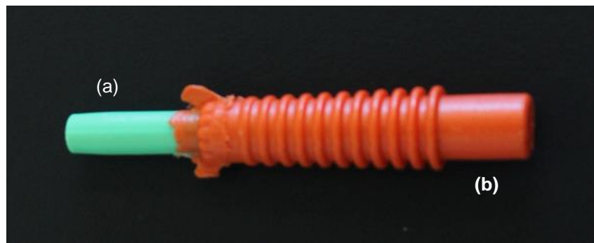
Figure 8.9: Shock tube holder (a) and main body (b) interface
