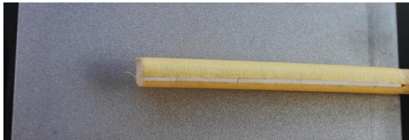
Figure 7.15: Reference RXKF charge on top of witness plate
