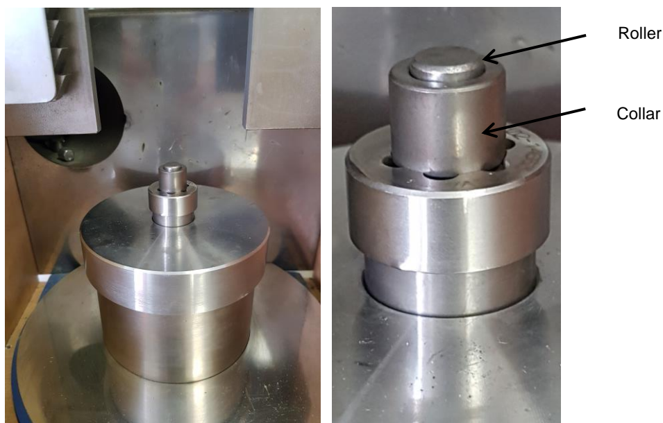
Figure 4.35: Collar and roller set-up
