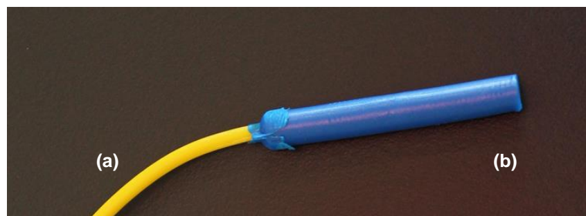
Figure 8.7: Shock tube (a) and shock tube holder (b) interface
