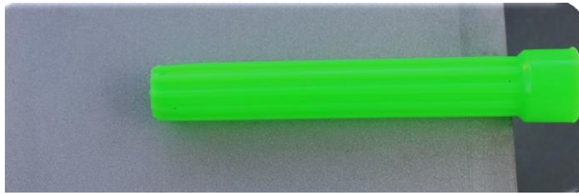
Figure 7.13: Filled booster casing on top of aluminium witness plate
