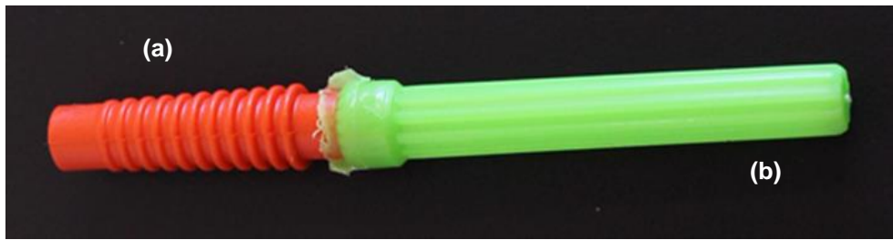
Figure 8.11: Main body (a) and booster (b) body interface
