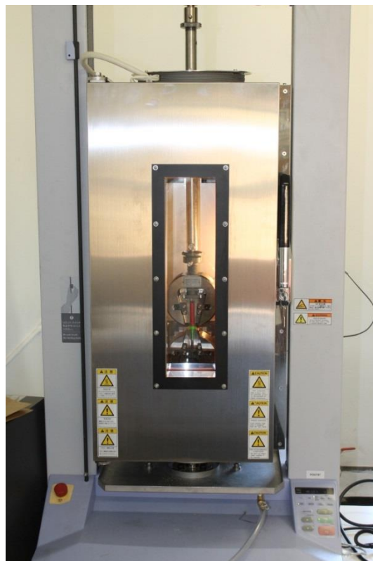
Figure 8.3: Sample inside climatic chamber on tensile tester
