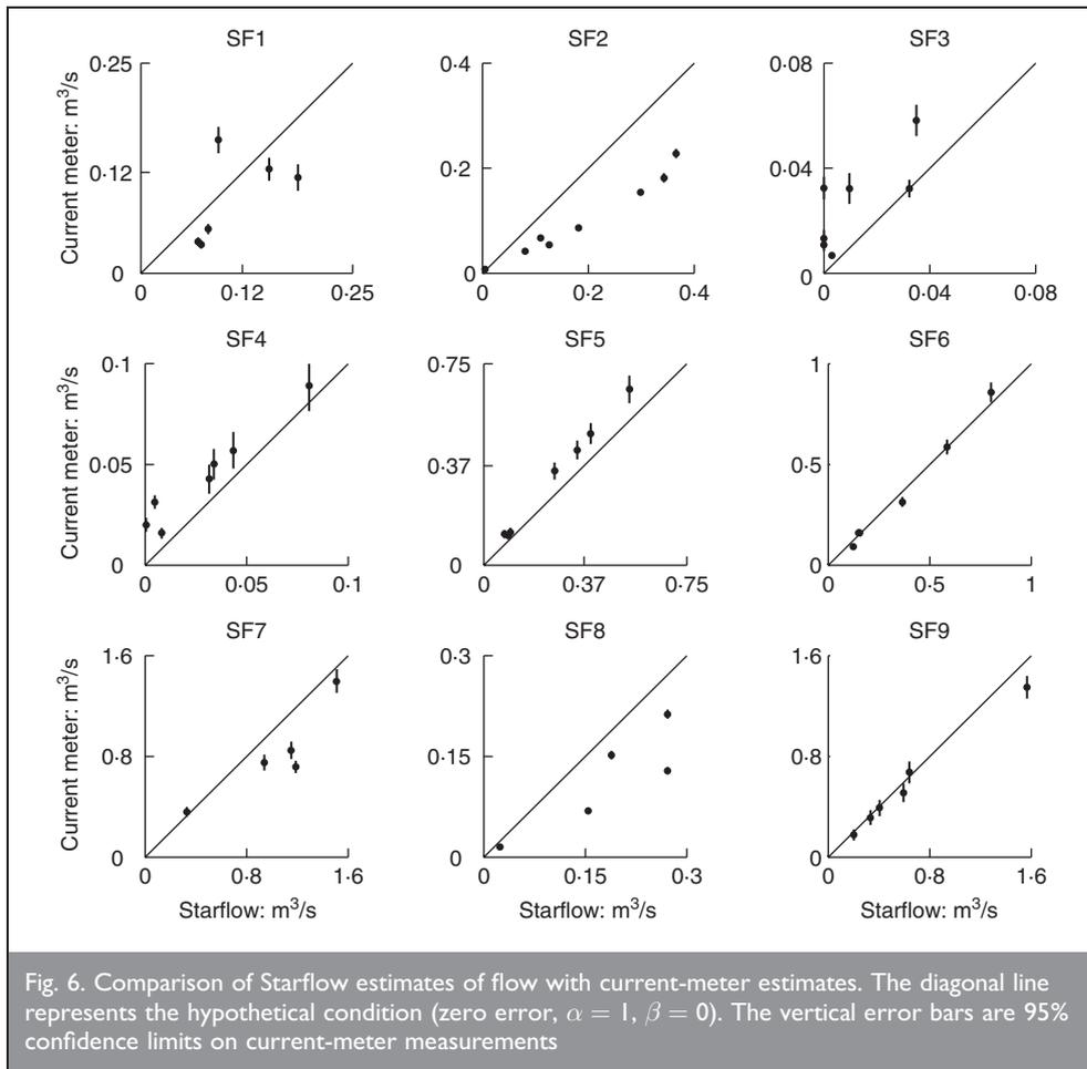
sample of flow at SF1 and SF2 is unknown). The Starflow calculations for SF1 and SF2 were adjusted on the assumption that either the initial or the final depth–area relationship applies to each depth and velocity sample.
