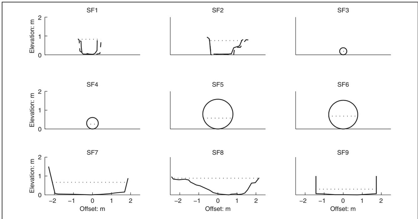
Fig. 3. The cross-sections at the nine sites (SF1–SF9). The Starflow in each case is located at offset = 0. The solid lines for SF1 and SF2 show the section shape as measured in October 2005, and the dashed lines as measured in March 2007. The dotted lines show the maximum water level over the period of Starflow operation
