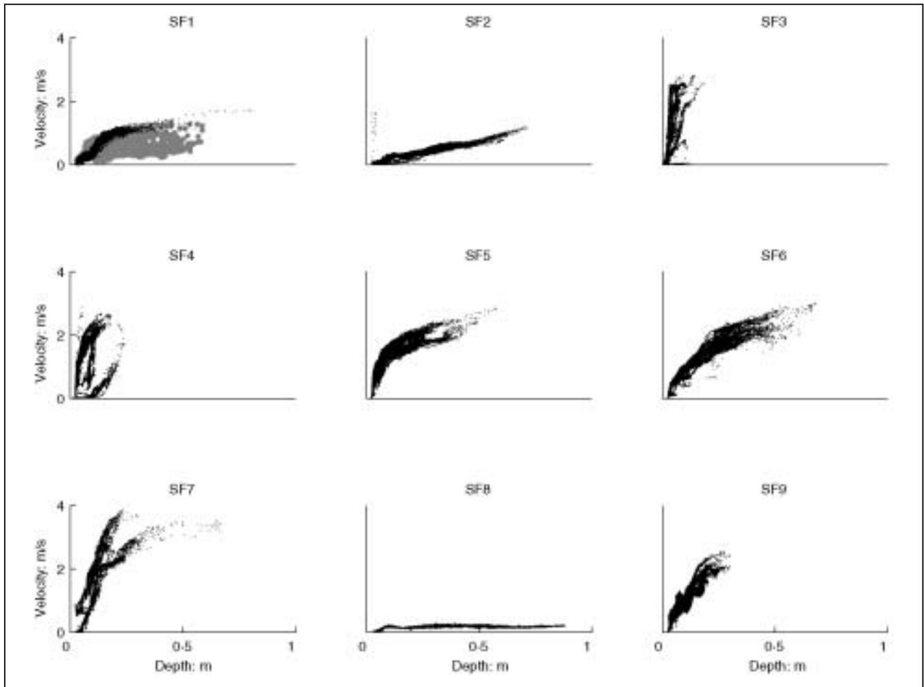
Fig. 5. Depth–velocity data for the nine sites. For SF1, the lighter shade represents data collected after July 2006
