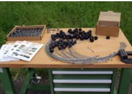
Passive RFID seals fabricated for the Smart and Secure Trade Lanes (SSTL) pilot project.
