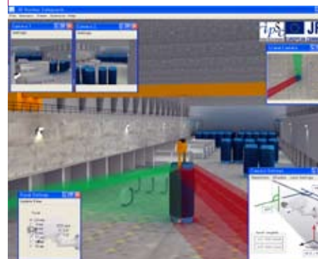
Safeguards Simulation Tool - Analysis of blind surveillance areas (from 2 cameras)
