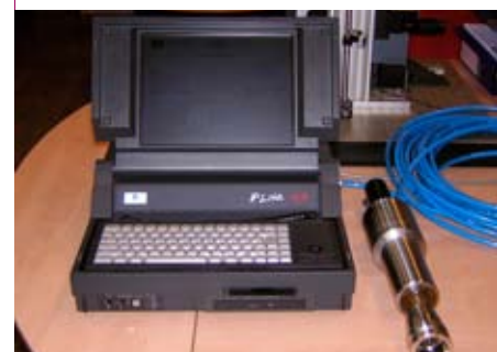
Last generation of sealing system for dry storage applications (seal, reading head & acquisition system)
