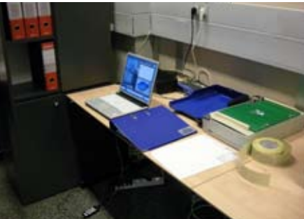
Management of classified documents (bookshelf, tagged folders, database, tagged sheets, tags, scanner with reading RFID antenna, document tray with RFID antenna)
