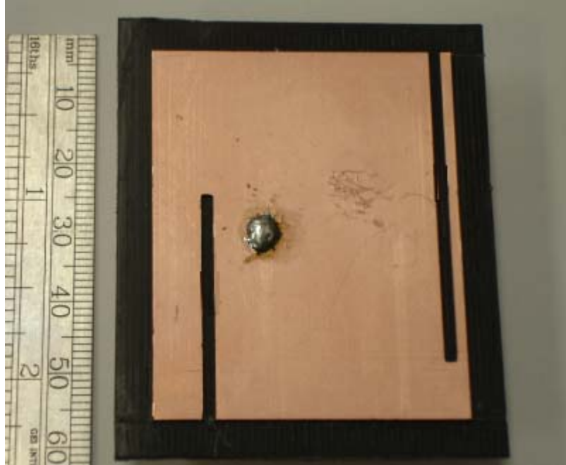
Figure 4.3: Fabricated bottom MSA with two slots when SW1 and SW2 are OFF.
