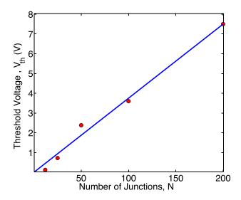
FIG. 10. Variation of the threshold voltage [obtained from Fig. 7(b)]  $V_{th}$ , as a function of the number of junctions N along the chain. A linear behavior as has been observed in several experimental studies. <sup>12,13,22,24</sup>
