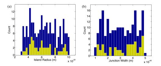
FIG. 6. (a) Distribution of radii of the islands along the chain of 50 junctions (yellow/light) and 200 junctions (blue/dark). (b) Distribution of widths of the junctions that couple the neighboring islands and through which the electron tunneling takes place. The 200-junction chain contains more large-width tunneling junctions, which play a dominant role in determining the device characteristics.
