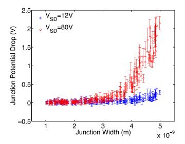
FIG. 11. Variation of junction potential drops with the junction widths in a chain of N = 200 junctions at two different source-drain biases  $V_{SD}$  [12 V (blue diamonds); 80 V (red circles)], as in Fig. 9. Error bars about the mean values show the standard deviations in the junction potential drops (over 5000 Monte Carlo steps, corresponding to approximately 1 ns at 12 V and 18 ps at 80 V) after the system has reached a steady state.
