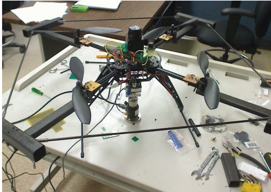
Figure 5.11: UAV sitting on force and torque sensors.
