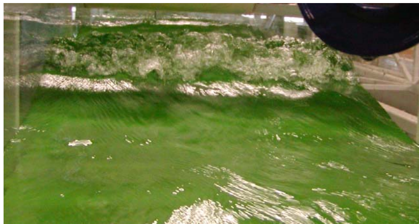
Fig. 6 – Undular surge with some breaking, Run 60-1. Lateral view (above) and looking downstream at the incoming wave crest (below)
