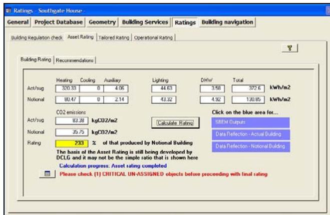
**Figure 6 SBEM rating for VRF air-conditioning system only**
