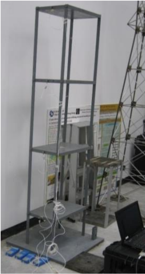
(a) Shear building model.
