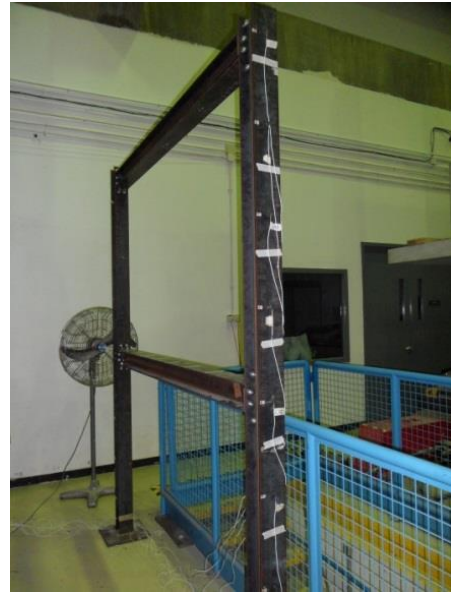
(b) Steel frame under wind load.
