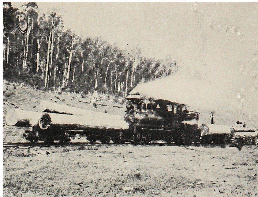
5. A three-cylinder Shay locomotive. The original one used, of 16 tons, had a T-shaped horizontal boiler, with a two-cylinder vertical engine set outside the main frame in the middle of its length. The crankshaft was extended fore and aft by an articulated shaft which was geared to a large mitre gear on each bogie wheel on that side of the loco, so the whole eight wheels were drivers. As they carried the whole weight of the engine and gear on one side the boiler was set out of centre towards the other side. This gave it a comical, Emmett-like appearance when viewed from the front. Seen rounding a curve it looked even funnier for the crankshaft was parallel to the centre-line, the bogie gear shafts tangential to the rails, and the sliding universally-jointed shafts connecting them at yet another angle! Subsequently the company owned an 18 ton two-cylinder model, and then this 24 ton three-cylinder model, the bell of which is now at Binna Burra. A two-cylinder Shay is illustrated in photograph 8.
