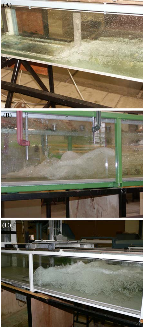
Fig. 5 Photographs of air bubble entrainment in hydraulic jumps for V_1/\sqrt{gd_1} = 5 (flow from left to right) (a) V_1/\sqrt{gd_1} = 5.1 , \rho_w V_1 d_1 / \mu_w = 2.4E+4 , x_1 = 0.5 m, W = 0.25 m (shutter speed: 1/60 s) (b) V_1/\sqrt{gd_1} = 5.1 , \rho_w V_1 d_1 / \mu_w = 3.8E+4 , x_1 = 0.5 m, W = 0.5 m (shutter speed: 1/40 s) (c) V_1/\sqrt{gd_1} = 5.3 , \rho_w V_1 d_1 / \mu_w = 7.1E+4 , x_1 = 1 m, W = 0.5 m (shutter speed: 1/80 s)
