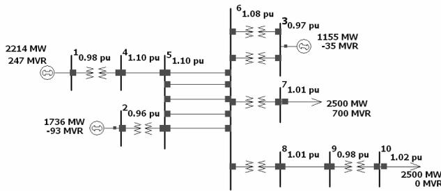
Figure 3 10 Bus BPA test System
