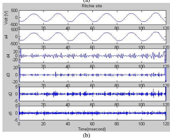
**Figure 13** Voltage sag disturbance, (a) 22:35:29 (b) 22:35:30
