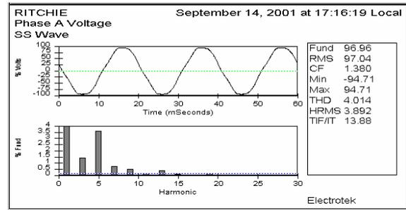
Figure 10 Steady-state waveform on phase A voltage
