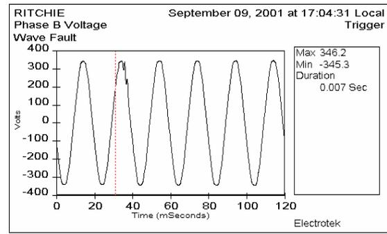
Figure 5 Low frequency oscillatory transient (2) Short/long duration variations
