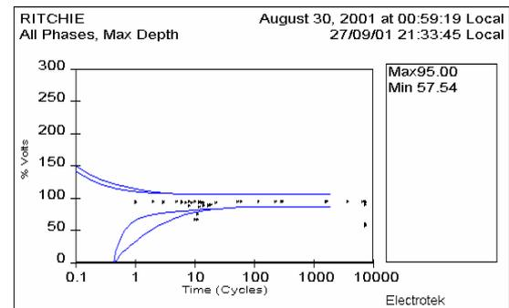
Figure 6 The CBEMA curve, showing the fatal sags
