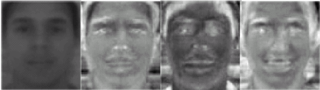
Figure 1. Typical set of eigenfaces as used for face recognition. Leftmost image is average face.
