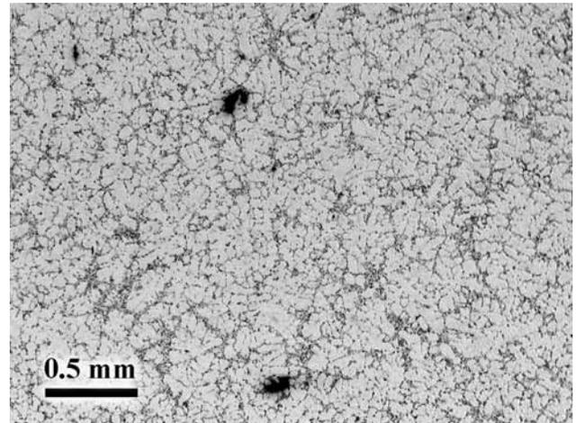
Figure 4: Microstructure of the gravity diecasting
