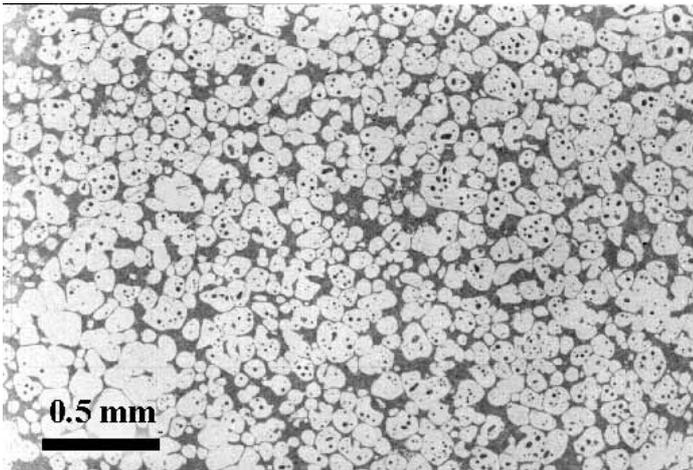
Figure 3: Microstructure of the semisolid casting.
