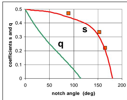
**Figure 5.** The predicted size coefficients for notches in timber beams; the plotted data points are taken from the slopes of the graphs shown in Figure 4.
