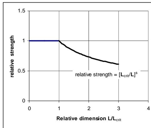
Figure 2. Illustration of the concept of the size factor.
