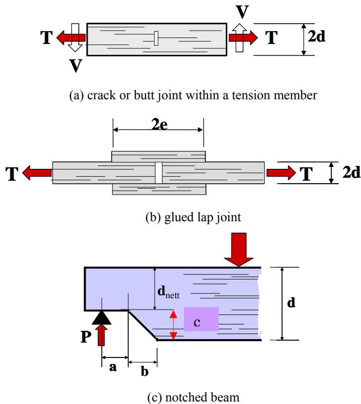
Figure 3. Examples of notches considered in AS 1720.
