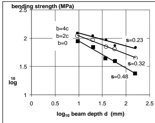
**Figure 4.** Measured bending strength of messmate (*E. obliqua*) for beams noted as shown in Figure 3c.
