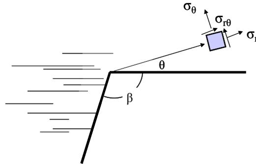
**Figure 1.** Notation used at a notch root with an included angle,  $\beta$
