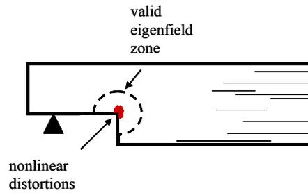
(a) Conditions in a structural member just prior to fracture
