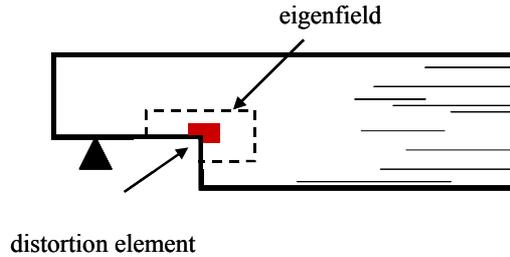
(b) Eigen field and distortion element used for computing stress intensity factors
