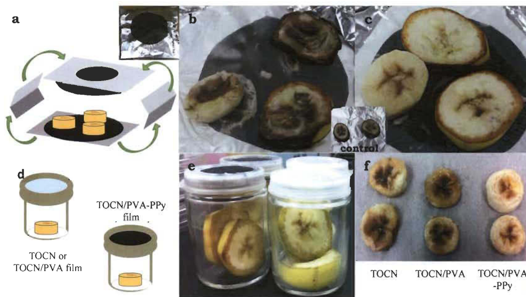
Figure 11.6 Schema of food packaging test by contact (a); food simulation after 5 days, with TOCN film (b), TOCN/PVA-PPy (c); schema of food packaging test by noncontact (d); food simulation flasks (left: TOCN/PVA-PPy and right: TOCN/PVA films) (e); piece of banana after 5 days (f)
