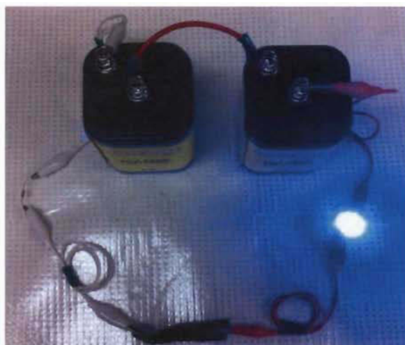
Figure 7.6 Demonstration of conductivity of p(PyCNFo) by light-emitting diode (LED)
