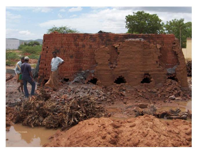
**Figure 17. Baked bricks with** *Prosopis* **roots used for the burning process.** (Photo: Kurt Walter).
