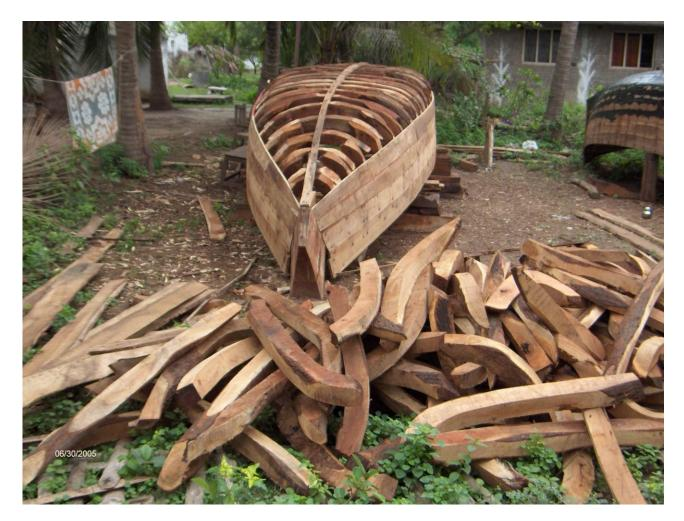
**Figure 18. Boat construction in Sitarampuram, using** *Prosopis* **wood.** (Photo: Kurt Walter).
