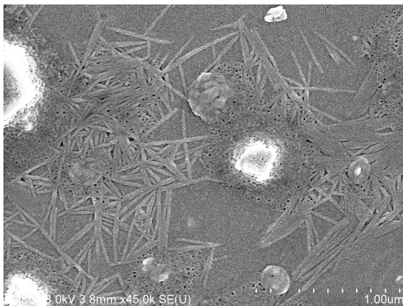
Figure 40. SEM image of chlorophyllcellulose fibres prepared by electrospinning from 25% (w/w) DMSO solution.
