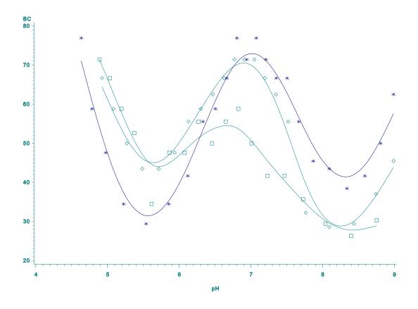
Fig 1. Buffering capacity curves obtained with different dilutions.
