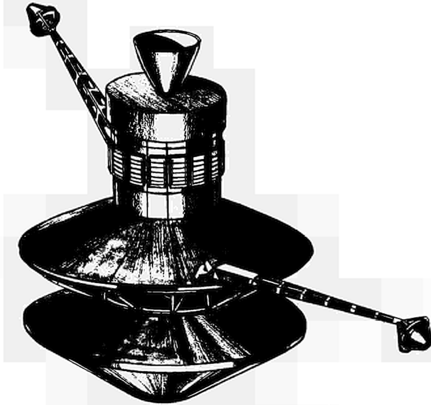
Figure 6. Voyager Spacecraft Concept with Isotope Thermionic Power System
