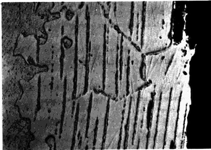
Fig. 2 Detail of a Mo can filled with ZrC and pyrocarbon-coated particles after 10 hours at 2000° C. ( x 250 )
