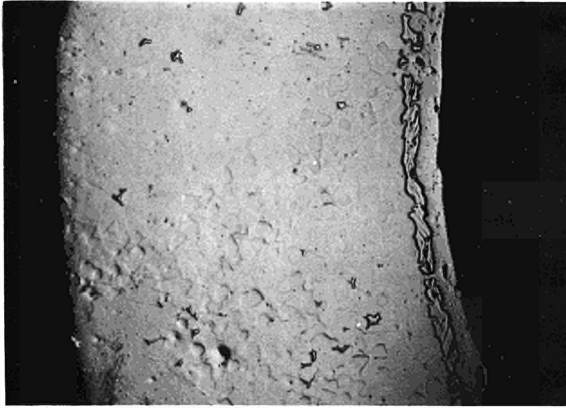
Fig. 7 Detail of a molybdenum can filled with AlN powder and pyrocarbon-coated particles after ten hours at 2000°C. (x29)
