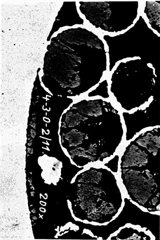
Fig. 5 Interface fuel-Mo (Section of fig. 4, unetched, 200 x)
