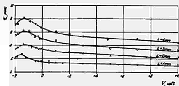
Fig.1. - The oscillation period dependence on the voltage and the interelectrode gap for \omega = 0,5 .
