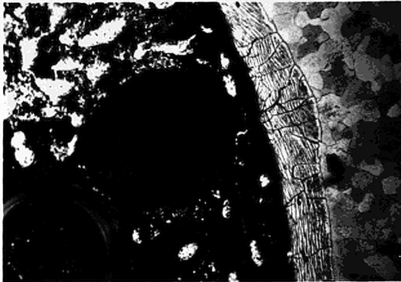
Fig. 6 Detail of a W can filled with TaC powder and PyC-coated uranium carbide particles after ten hours at 2000^{\circ}\text{C} , showing the influence of the proximity of a particle. (x75)
