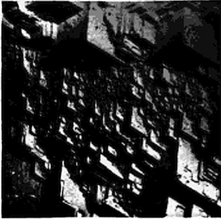
Fig. 1 Electron micrograph of a replica of an etched tungsten-{111}-surface, 2500 x
