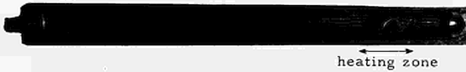
Fig. 1 - Failure of Ta/Li heat pipe by impurity corrosion (9 hours of horizontal operation at 1600°C, heating rate 155 w/cm 2 )
