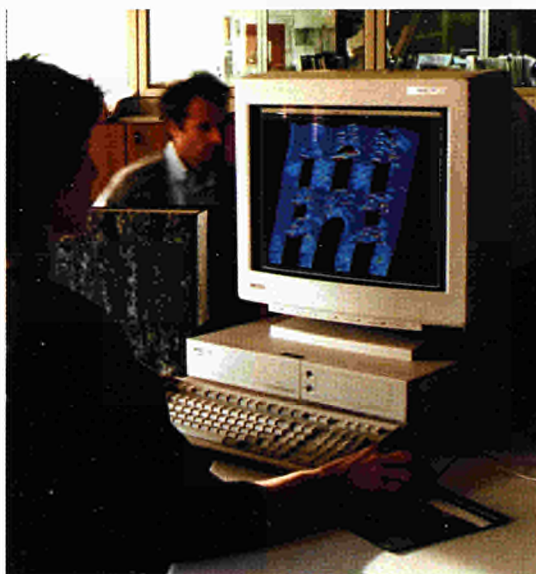
Figure 5.4: Computer simulation (displacement and damage patterns) expected during a seismic event on the Palazzo Geraci allowed to set up the test parameters. It is hoped that computer simulations will help predict earthquake behaviour of similar historical buildings
