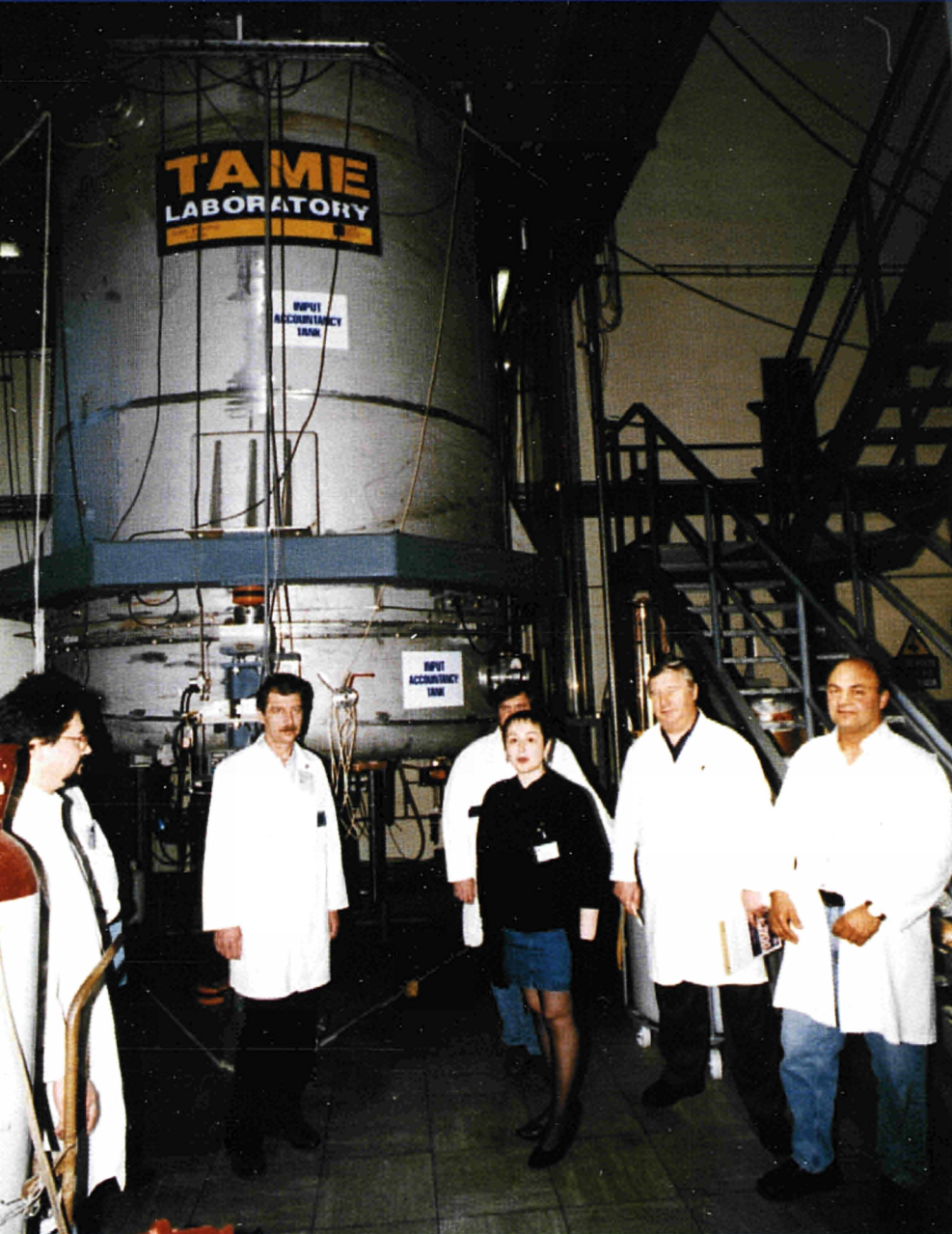
Figure 2.1: Mass and volume measurement inspection techniques, optimised in the TAME Laboratory have been applied to olive oil storage tanks. The methods were demonstrated in-field at an olive oil tank storage facility in Fasano, near Brindisi (Southern Italy). The dedicated system, which involved lowering a measurement probe in a controlled manner into the tank, showed that it was feasible to detect the difference between two olive oils via density difference. Aim of this activity, performed on behalf of DGVI, is to provide national inspectors with a means of detecting fraud in the case of claims for certain subsidies related to olive storage declarations. (author: B. Hunt)
