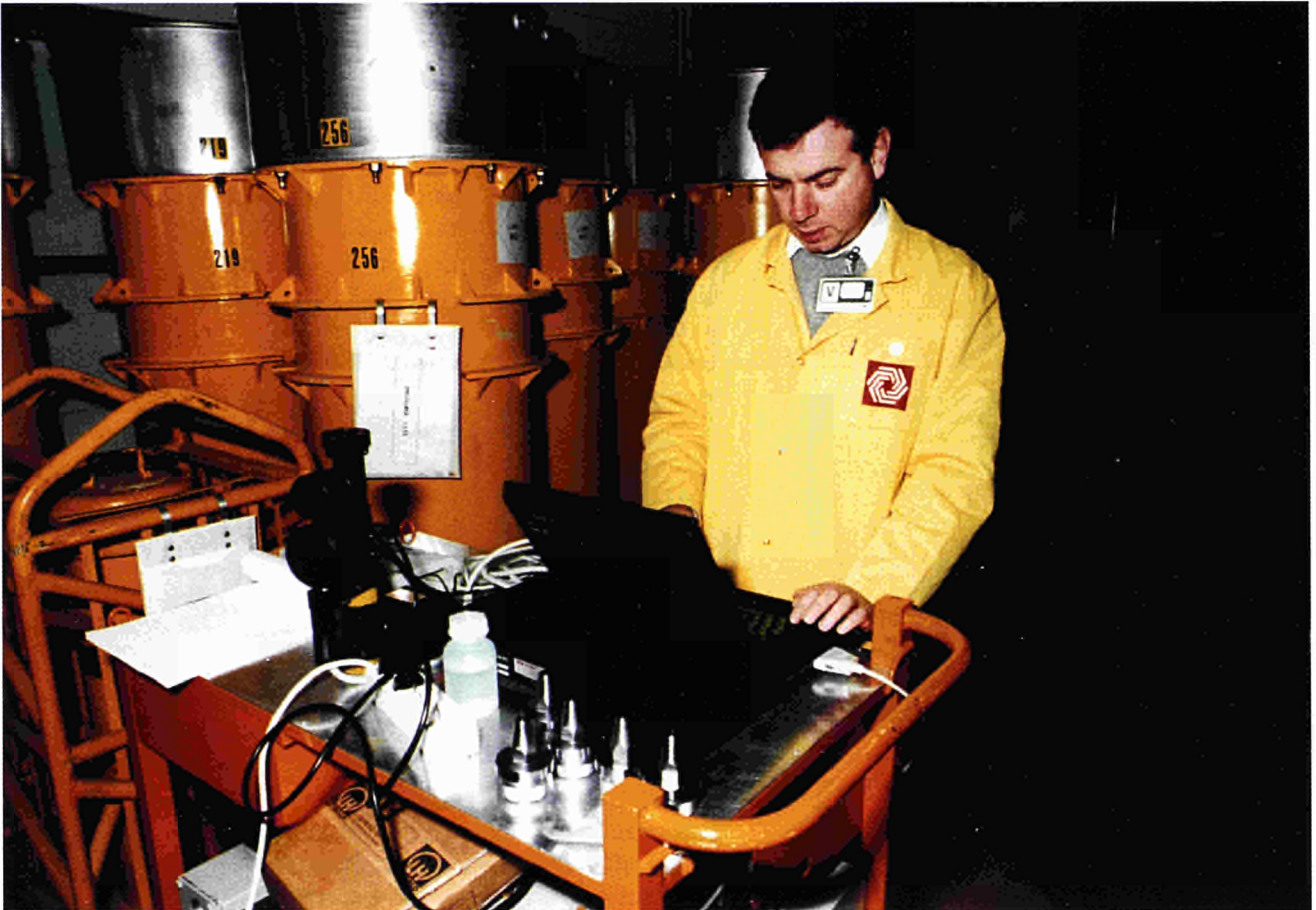
Figure 9.3: (a) Transport test for special safeguard seals. Preparing to install a special safeguards seal on a PuO 2 transport container at Cadarache (FR).
