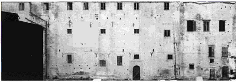
Figure 5.5: Steri building complex: Jail building orthophoto. An orthophoto is a map-like photograph that has a constant magnification scale. It is an orthogonal projection of the scaled original object
