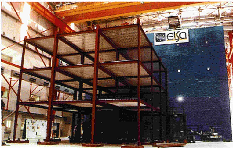
Figure 6.3: A typical three-storey steel frame construction was tested in ELSA. The scope was to verify the Eurocode 8 on earthquakes
