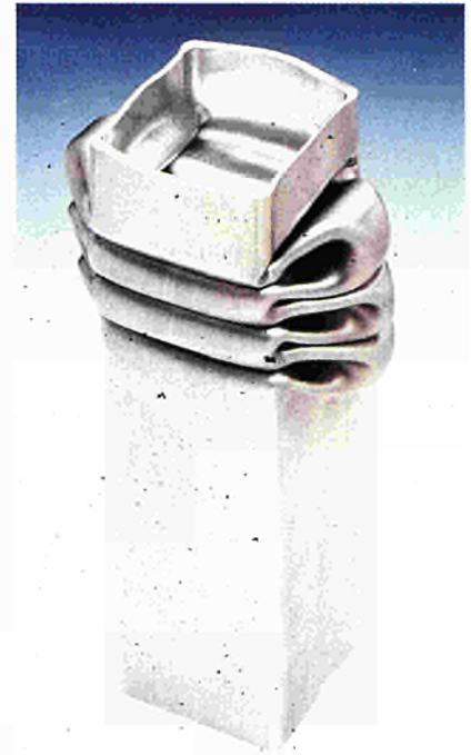
Figure 4.4: The Large Dynamic Test Facility (LDTF) method is the only method available which can measure the complete deformation/energy absorption history during a fast dynamic event. Configuration for compression tests serves to measure longitudinal elements as used in cars during a collision as shown in the photograph. The LDTF facility is shown in Figure 6.5
