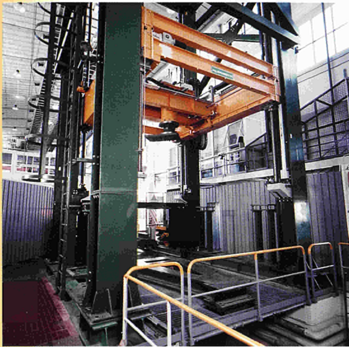
Figure 10.2: ROBERTINO heavy robotics facility: a big, 4 degrees of freedom, gantry robot for the experimental validation of the Remote Handling devices and procedures to be used for the "Next Step" Fusion Reactor maintenance as well as for industrial applications
