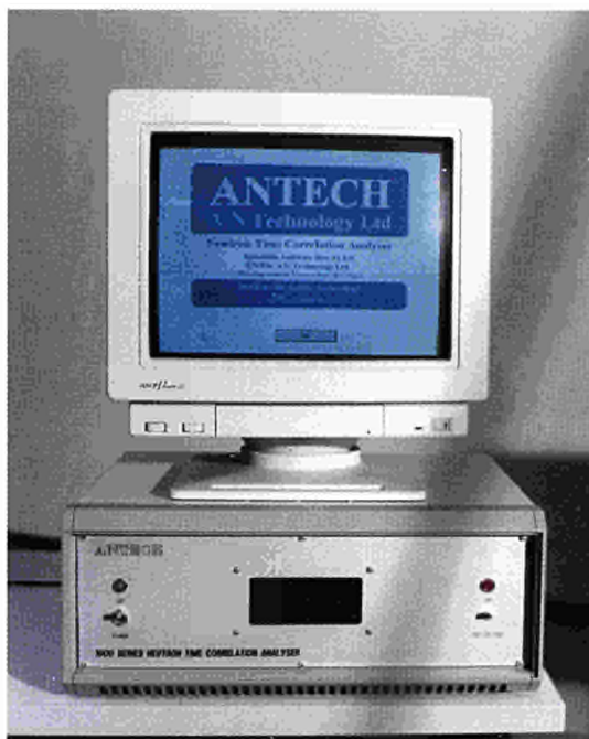
Figure 14.2: The ANTECH Series 1000 Neutron Time Correlation Analyser for Multiplicity Counting allows improved non-destructive measurement of Plutonium. It is a result of JRC's safeguards research and recent implementation efforts by ANTECH as part of the technology transfer process.
