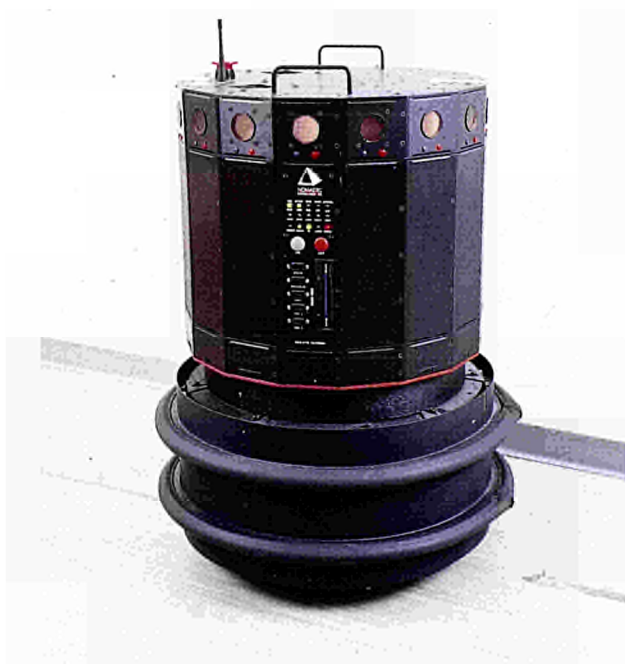
Fig. 3.3. TESEO: the test robot used for reinforcement learning navigation. The hardware is a commercially available Nomad 200 mobile platform
