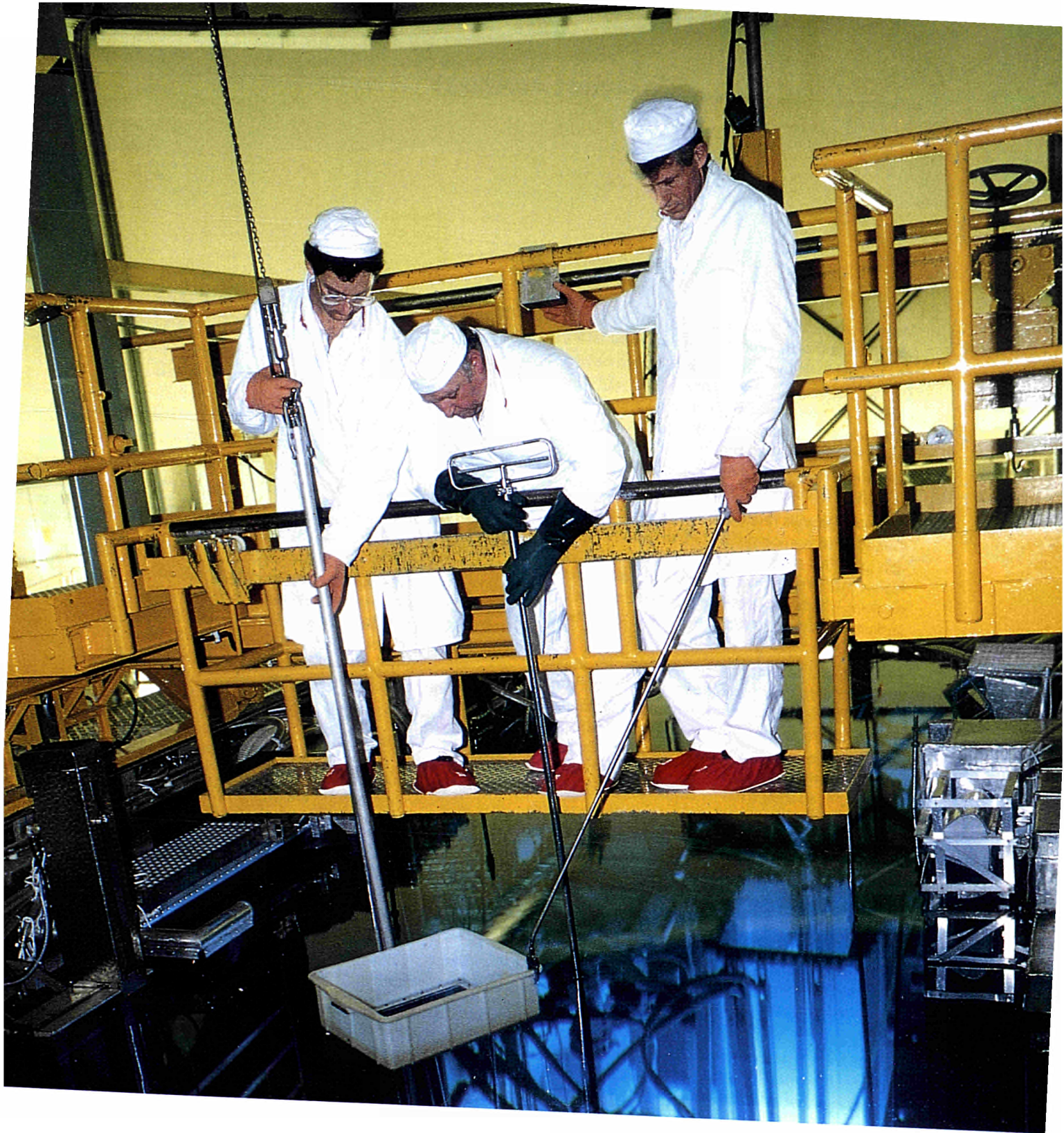
Above: Unloading of irradiated U 235 samples from a core position
