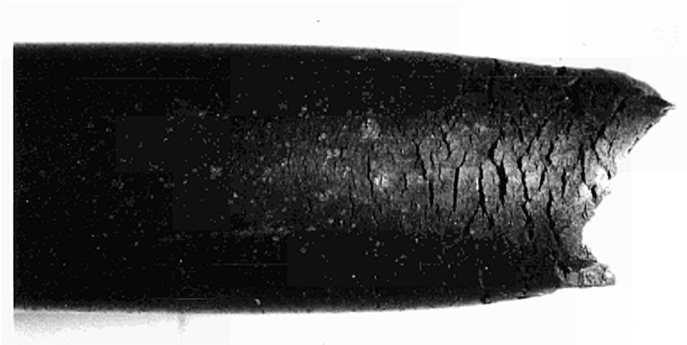
Fig.4: Extensive secondary cracking of the 15 MnNi 6.3 steel tested in Q-brine at 170°C, 13 MPa and 10^{-5} \text{ s}^{-1}
