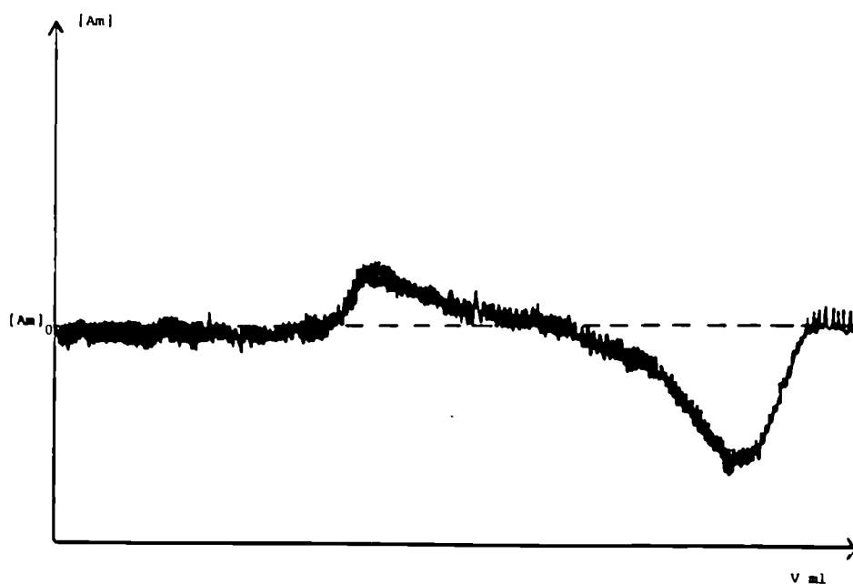
Figure 2 : Chromatogramme obtained on G25 with the system Am(III)-Aldrich humic acids (same conditions as in Table 2)
