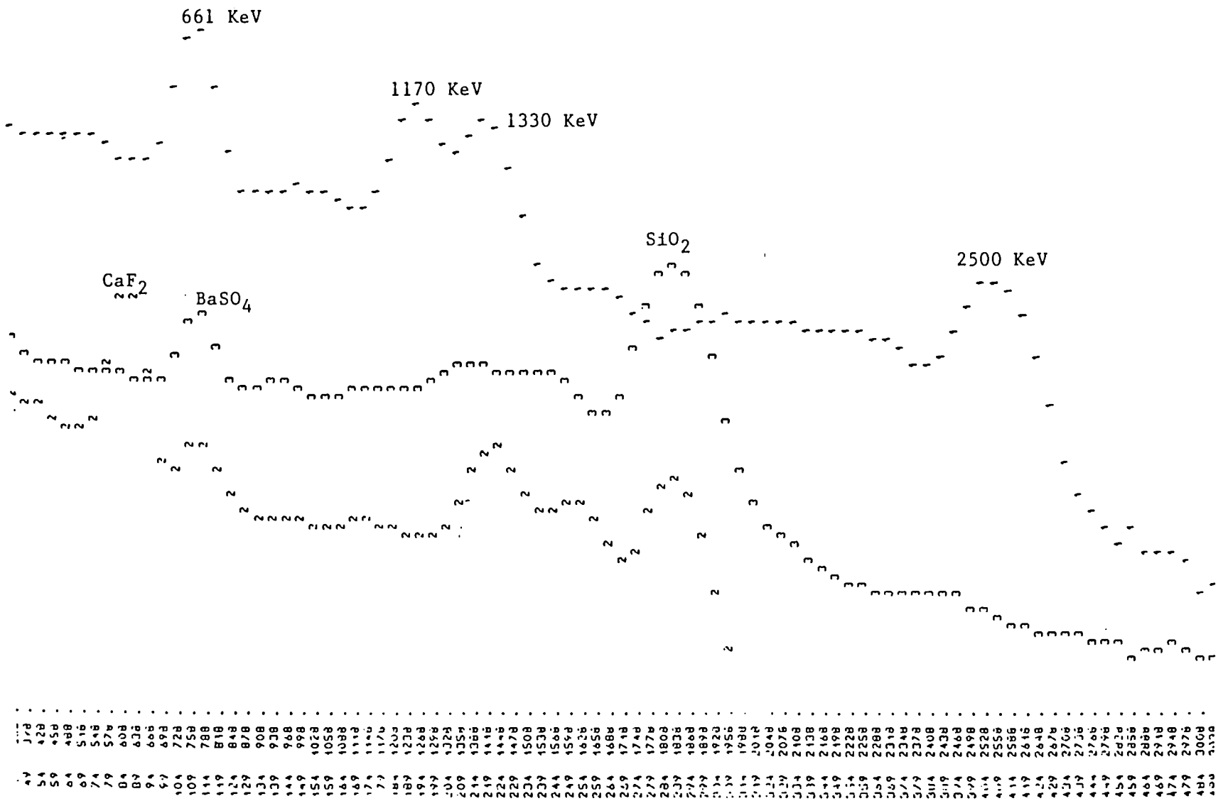
Fig. 2 - Gamma spectra of calibration standard CoCs(1), concentrate (2) and tailing (3) of fluorite.
