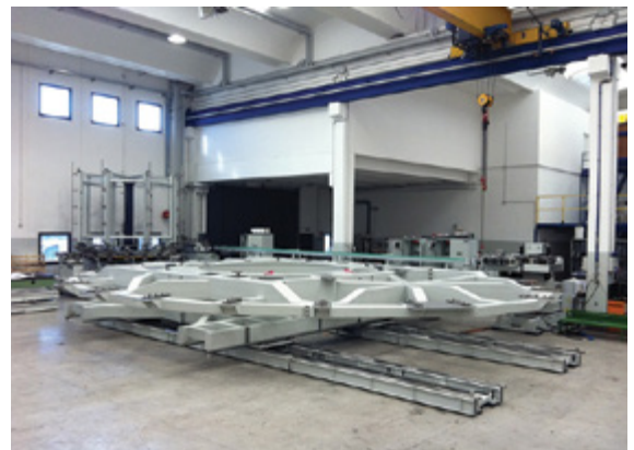
The winding line for the Double Pancakes (courtesy of ASG and TPA)
