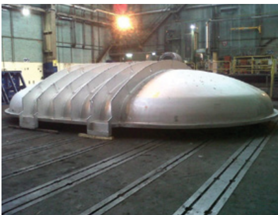
TF Coil Test Facility Cryostat under construction - closure lid (left) and cryostat tank (right)
