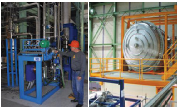
Left: European Breeder Blanket Test Facility (EBBTF) at ENEA/Brasimone (Italy) and its new Helium turbo circulator able to reach TBM full-scale prototype testing
