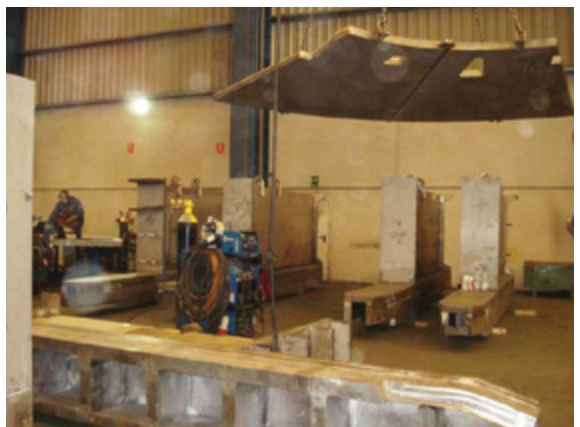
Cryostat Base Manufacturing - advanced stage of radial legs preparation
