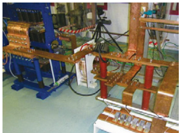
QPC - Test of the By-pass switch prototype at RFX (Padova, Italy)
