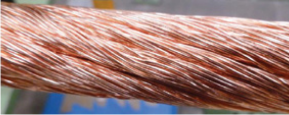
Superconducting cable - external appearance of cable produced for tests at the Sultan facility
