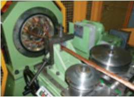
Left: Superconducting cable - final cabling; Right: TF Conductor - jacketing line
