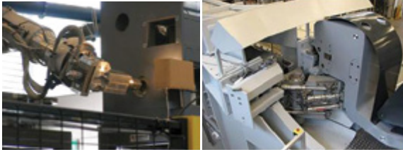
Left: Bolting tool operating the cassette locking system Right: Trials measuring the robustness of the RH equipment when removing divertor cassettes in off-normal conditions
