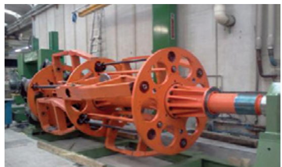
TF Conductor Cabling Line - new machines for final cabling stage
