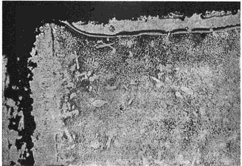
Structure of the surface zones of SM 200 after a corrosion test at 1,100°: left, vertical, chromium-aluminized zone; horizontal, unprotected zone (note the deep scoring along this zone)
