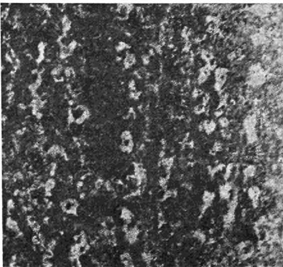
Standard plates for corrosion testing of metallic coatings — Anodic coating — Electrolytic nickel deposit on steel subjected to the salt-spray test (PN X 41-002)
