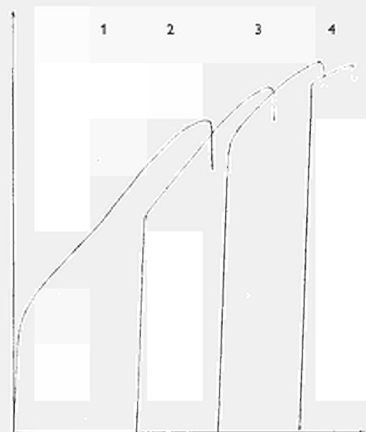
Some conventional stress-strain curves for superhardened cold-drawn wires (Austenitic stainless steel C = 0.63%; Ni = 8.1% Cr = 18.1%)
