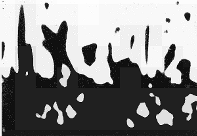
Electron image of the metal/enamel interface (4,000 : 1)
