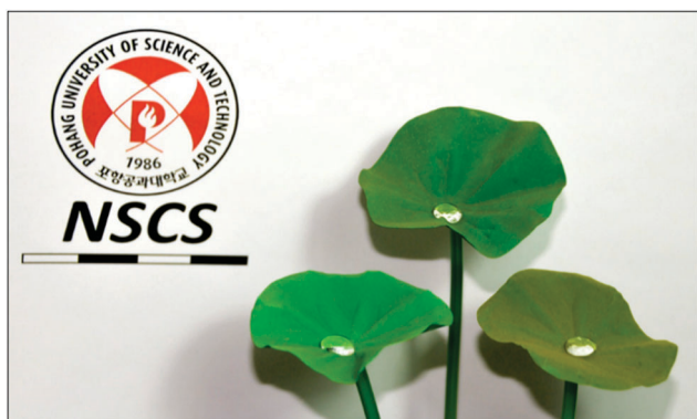
Fig. 7 Photograph of superhydrophobic artificial lotus leaves. The leaves were made of copper plates, and they colored by forming green patina and surface modification. Different colored surfaces could be obtained by controlling the reaction time of brochantite and surface modification. The scale bar corresponds to a length of 10 cm.
