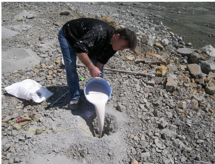
Figure 4. Application of plaster paste to hole collar
