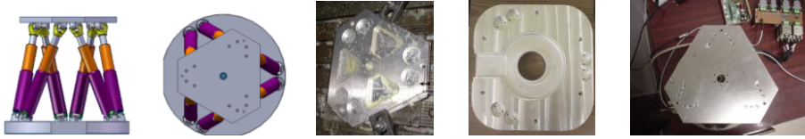
Figure 4. The solid models obtained from SolidWorks program and the plates manufactured on CNC machine.
