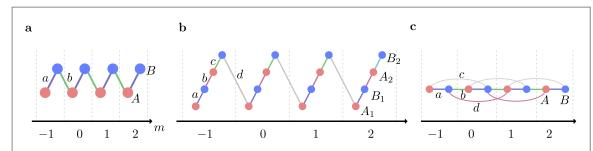
**Figure 1.** 1D chiral models. Sketch of the SSH (a), the SSH $_4$  (b) and the SSH model with staggered long range hoppings (c). Red and blue sites belong respectively to the A and B sublattices, thin lines denote hoppings, and the unit cells of the lattice are indexed by the integer m. The corresponding Hamiltonians are explicitly chiral, as these contain no term coupling a sublattice directly with itself.
