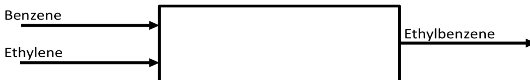
Figure 1. Process concept diagram of the ethylbenzene process. Inlet streams are benzene and ethylene; product is ethylbenzene (3).
