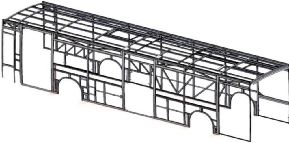
Figure 58 Cad model of bus body structure
