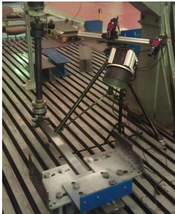
Figure 65 Stereo DIC equipment installation.
