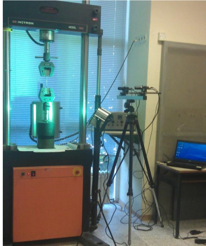
Figure 53 Tensile test setup
