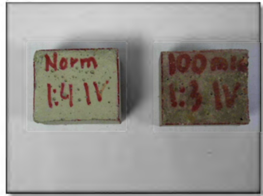
Fig. 9. Crystallization of salts.
