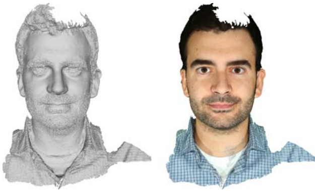
Figure 15: 3.4 million triangle 3D mesh acquired using Beeler's approach [BBB*10] and used for testing the performance of our algorithm.
