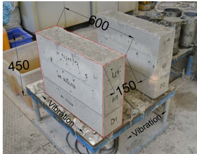
Figure 8-4: Vertical (UHD) concrete elements.
