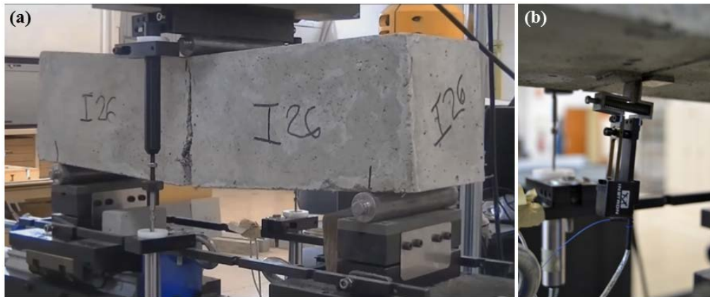
Figure 5-1: Three-point bending tests: (a) specimen while testing; (b) detailed view of the CMOD gauge that controls the test.
