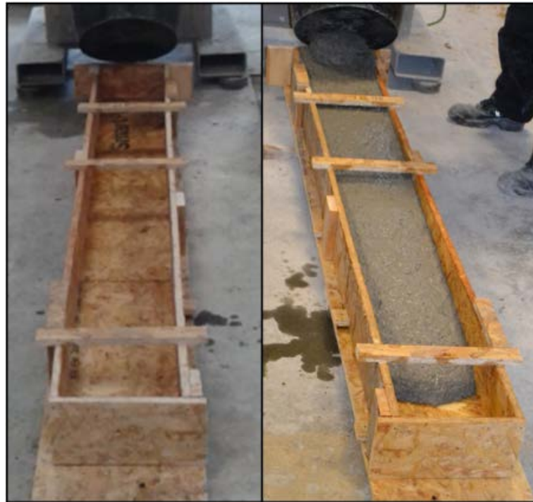
Figure 8-2: Long-beam formwork and pouring of SCC6-60.
