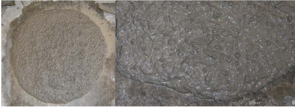
Figure 6-2: Visual appearance of the slump-flow spread of H1.
