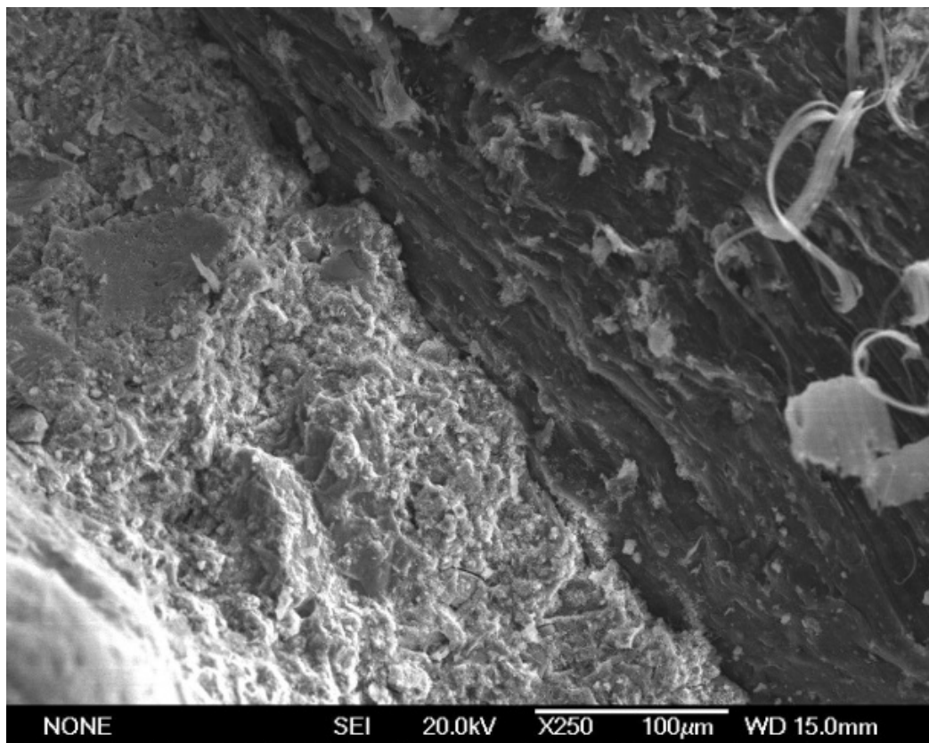
Figure 7-21: Interface between polyolefin fibre and cement paste.
