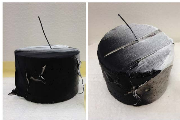
Figure 7-4: Visual aspect before testing of two specimens with embedded length 10 mm long and incidence angle 15 and 30 degrees.
