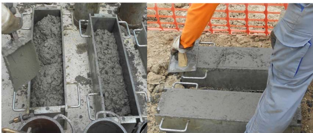
Figure 12-7: Filling of the moulds and levelling of the surface of the prismatic samples.
