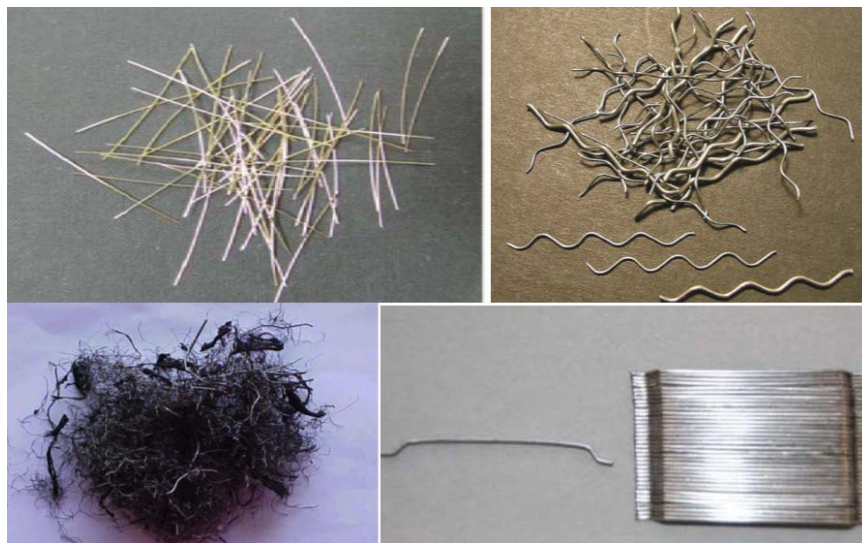
Figure 3-7: Several shapes and types of steel fibres (Banthia & Sappakittipakorn, 2007; Aiello, et al., 2009).
