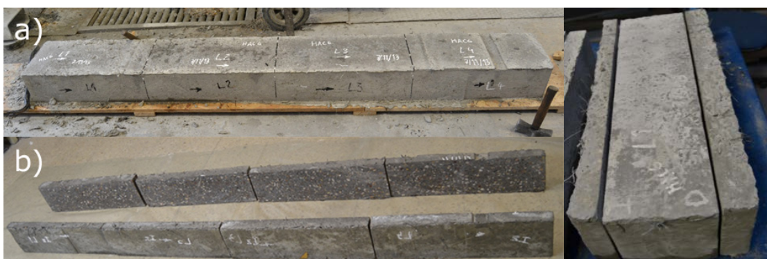
Figure 8-3: (a) Beam element after removing the mould; (b) sides removed from the concrete element to avoid the wall effect; (c) Sample L1 with the lateral sides removed.
