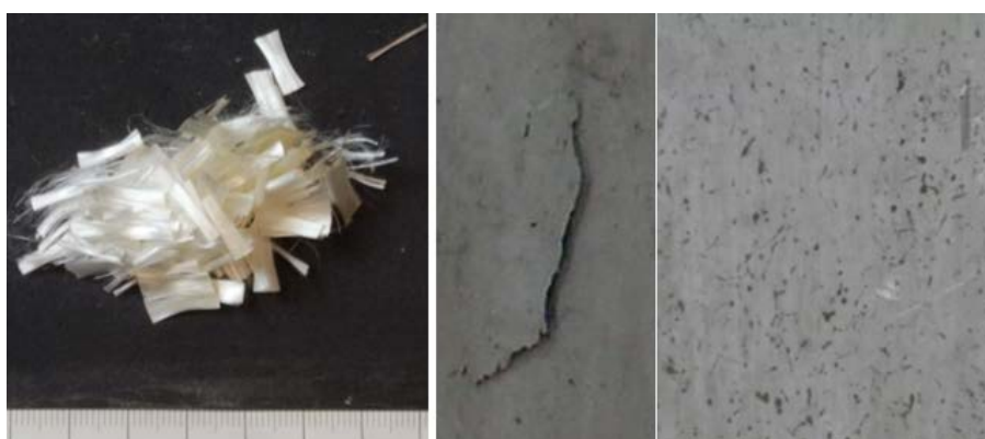
Figure 3-9: Typical micro-polypropylene fibres, fire spalling and water dots in concrete under fire resistance tests (Gálvez, et al., 2014).
