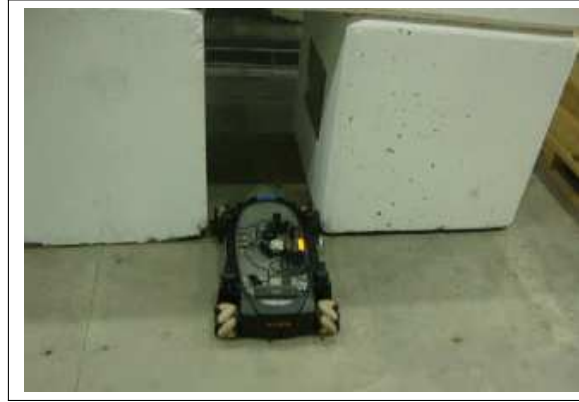
Figure 4.13: Thick reinforced concrete block used for tests.
