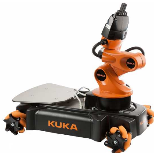
Figure 2.1: Design of the youBot mobile robot platform with arm. Source: youBot-stores GmbH.
