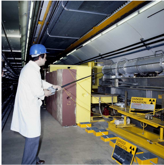
Figure 1.2: Radiation Protection (RP) personnel performing a RP survey manually.
