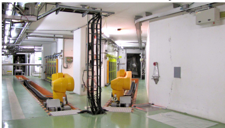
(b) A view of the ISOLDE target area showing the KUKA industrial robots for handling radiation targets.
