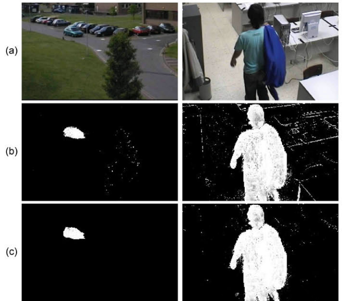
Fig. 7. Moving object detection with different spatial bandwidths in the background modeling. (a) Original images from two sequences. (b) Detections with \sigma_{\beta,H} = \sigma_{\beta,W} = 0.01 . (c) Detections with \sigma_{\beta,H} = \sigma_{\beta,W} = \sqrt{2}/3 .
