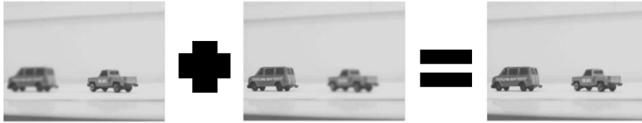
Figure 3.3: Fusion of two images with different depth of focus (extracted from [Pajares 2004]).
