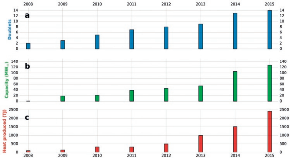
Figure 1.1 Number of doublets (a), respective installed capacity (b) and heat produced (c) for deep geothermal systems in the Netherlands. Source: (Bakema and Schoof, 2016; Ministry of Economic Affairs, 2016).
