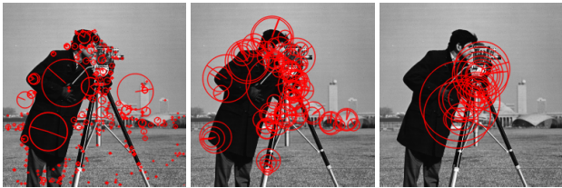
(a) Features detected by SIFT (b) Features detected by SURF (c) Features detected by ORB
