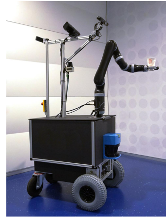
Fig. 6. The robot used for the experiments. The laser in the front of the robot is used for localization and obstacle avoidance. The two 3D sensors on both ends of the top bar are for 3D obstacle avoidance. The front sensor rotates based on the current speed of the robot to better detect obstacles.
