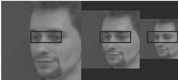
Figure 5: Searching for an eye-pair in different scales of width (54, 48, 33 pixels, respectively) with the same window frame. The best fit here is the middle one with an image width of 48 pixels. The resolution of the window frame (black rectangle) is 24x9.
