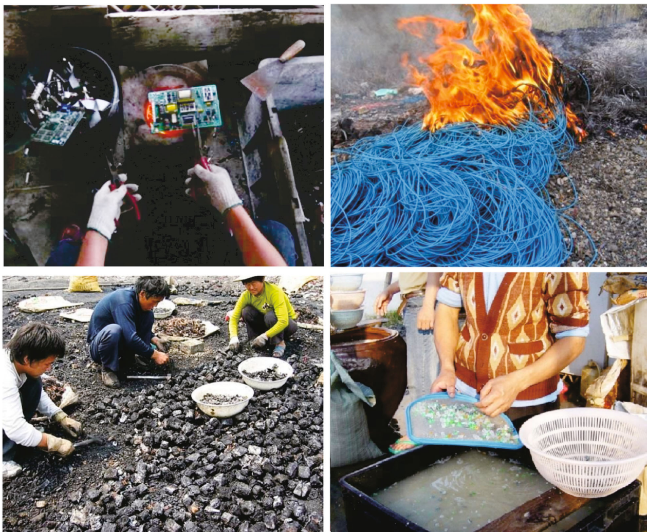
Fig. 1 Informal e-waste recycling activities in Guiyu, including roasting, burning, dismantling, acid leaching, inappropriate shredding, and dumping.
