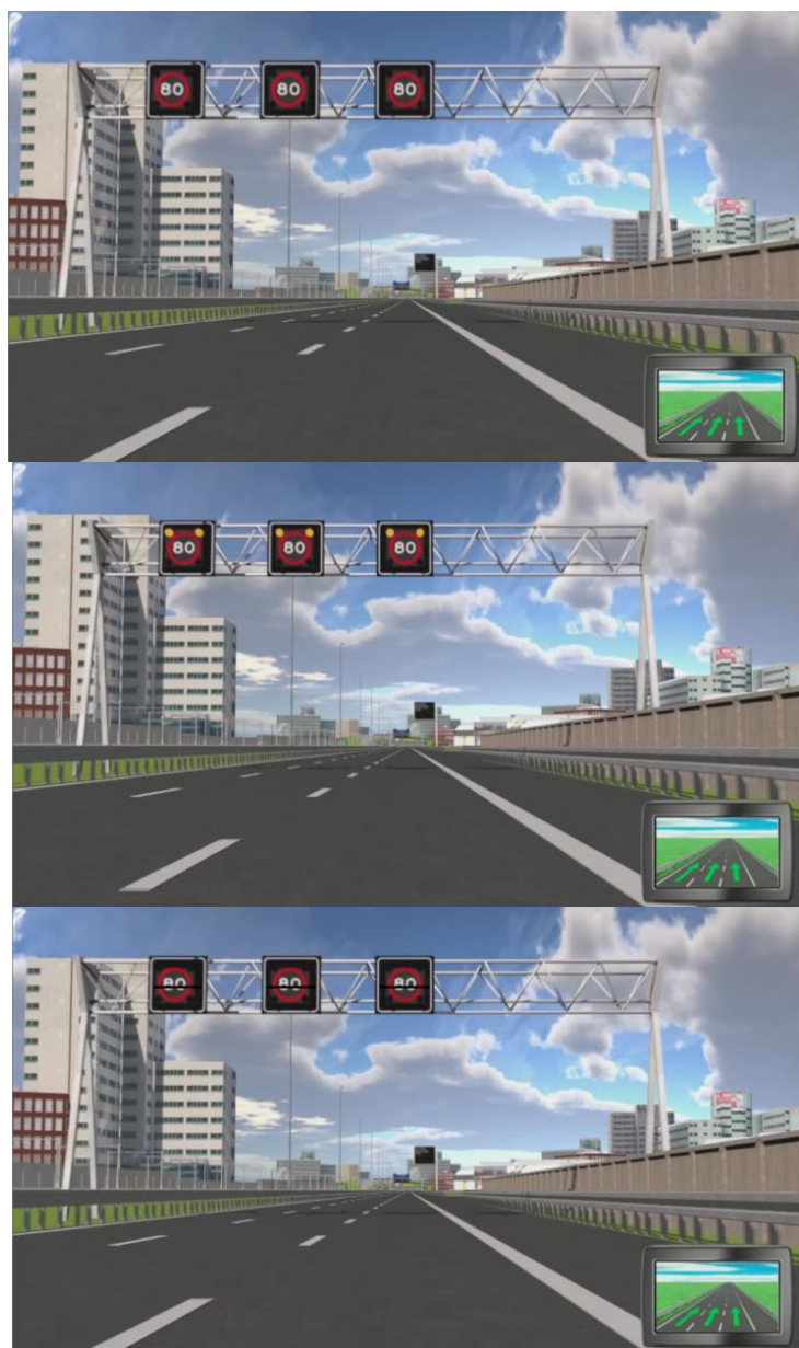
Figure 2. Screen shot of the second gantry under three conditions of information discriminability in video 14. From top to bottom: Basic, Flash, and Wave.
