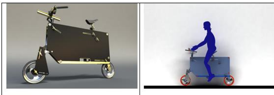
Figures 7-8 Measuring model. This prototype has been used to test different postures. All the components are adjustable
