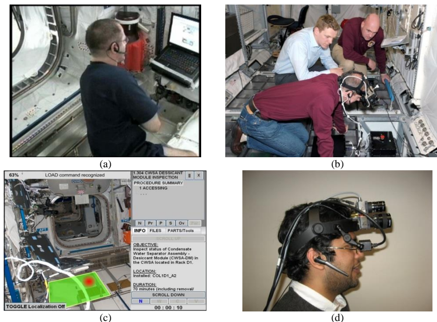
Figure 4 Clockwise from top-left: a) Astronaut Chris Hadfield testing voice recognition on the CRUISE experiment (credit: ESA/CSA); b) Astronaut Frank De Winne training to use the WEAR system (credit: ESA image archive); c) The WEAR head mounted procedure viewer; 4) WEAR user interface rendering procedures and guidance information using augmented reality
