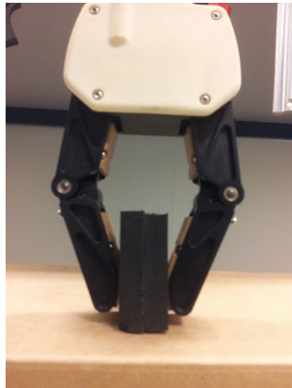
(d) Gripper grasping a compliant body as in (4.63).
