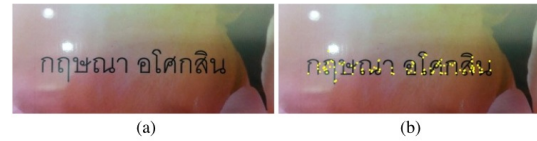
Figure 11: Extraction of characters from a background using object attention patches. (a) Original image. (b) Extraction of characters using character model attention patches.
