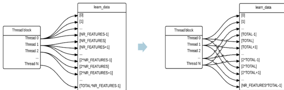
Figure 3. Transformation from uncoalesced to coalesced memory accesses.
